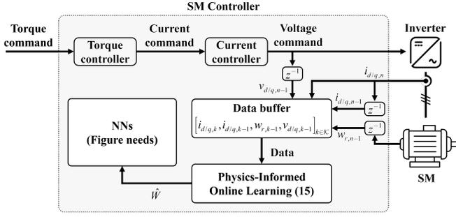
Fig. 1. Schematic diagram of the proposed physics-informed online learning method for the flux linkage model of SMs.
